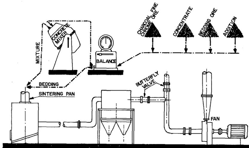
FIG. 01 - SCHEMATIC LAYOUT OF THE PILOT SINTERING PLANT
