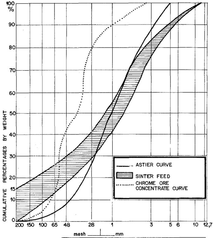
FIG. 05 - SINTER FEED, ASTIER AND CHROME ORE CONCENTRATE GRANULOMETRIC CURVE
