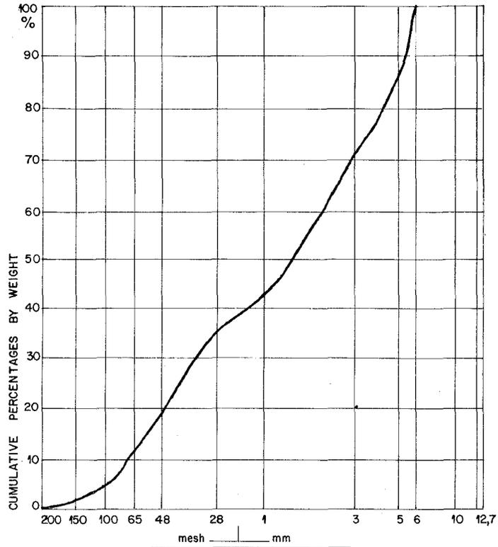
FIG. 04 - CHARCOAL FINES GRANULOMETRIC CURVE
