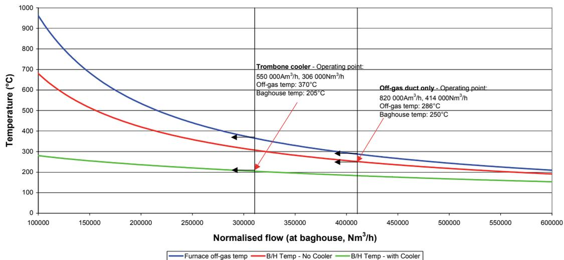
**Figure 3:** Comparison of Operating points – with / without Cooler
