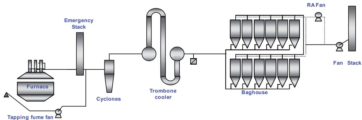
**Figure 4:** Gas cleaning system layout – Furnaces 45 to 48
