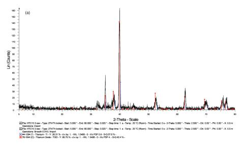
Figure 7—X-ray diffractograms of the, (a) planetary milled titanium powder and (b) roller milled titanium powder
