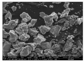
Figure 8—SEM micrograph of TiH<sub>2</sub> powder produced at (a) AG Materials Inc. [website: http://www.agmaterials.com/products/titaniumhydride.html], and (b) Mintek
