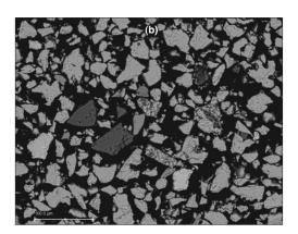
$\label{prop:control} \textbf{Figure 9--SEM micrographs of milled titanium hydride by (a) planetary mill, and (b) roller mill}$
