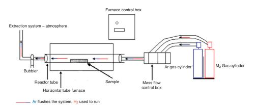
Figure 2—Schematic drawing of a horizontal tube furnace
