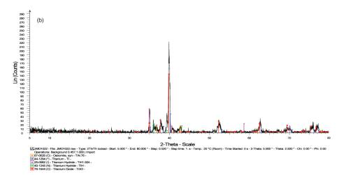
Figure 7 (continued)—X-ray diffractograms of the, (a) planetary milled titanium powder and (b) roller milled titanium powder
