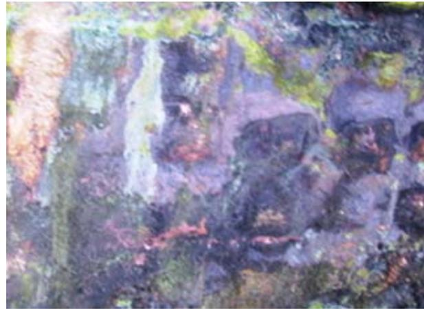
**Figure 7. Severely corroded, unprotected copper block. Black copper sulphide pervasive. Increasing evidence of green copper hydroxychloride in close proximity to copper**
