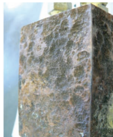
Figure 13—Copper corrosion at low 50°C temperature after only 5 days' exposure
