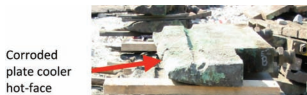
Figure 4—Severe upper plate cooler corrosion at Waterval Smelter. Note increased corrosion of upper plate cooler located in the furnace nearest the top of slag and concentrate interface
