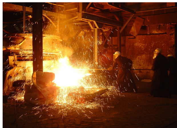
Fig. 2. Tapping the cauldron (pilot furnace) at Mintek (photograph by Geldenhuys, Mintek, 16 April 2004).
