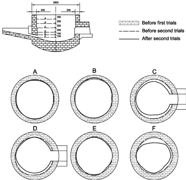
Figure 5: Refractory profiles before and after the two trials
