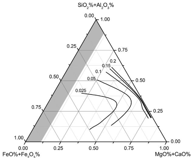
Figure 1: Iso-carbon lines in  $\text{SiO}_2\text{-Al}_2\text{O}_3\text{-CaO-MgO-FeO}$  system with  $\text{MgO}\%=8$
