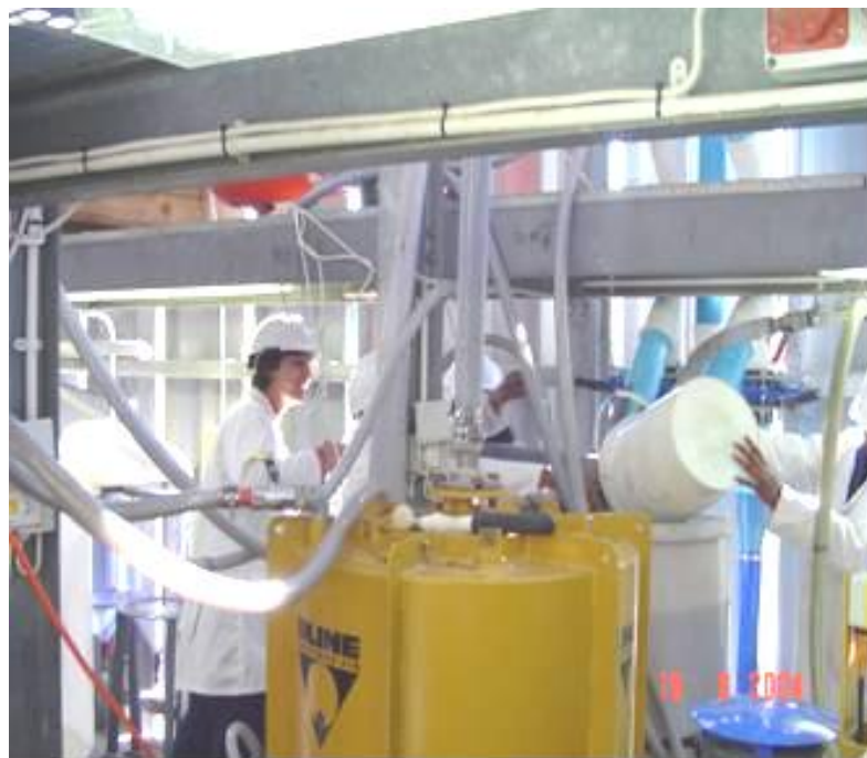
Figure 3: Students operating the in-line pressure jig pilot plant
