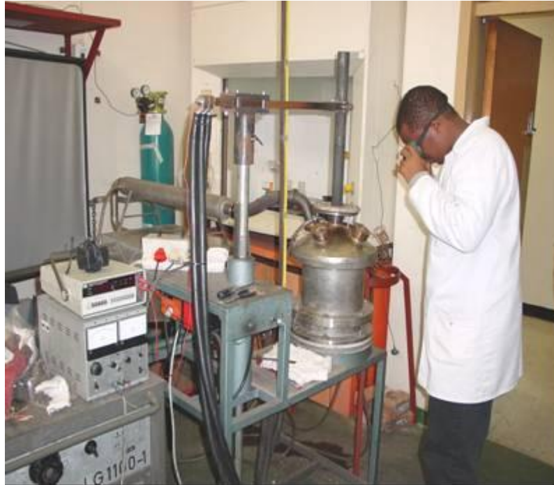
Figure 2: A student running the 60 kW DC plasma arc furnace for the smelting of chromite fines
