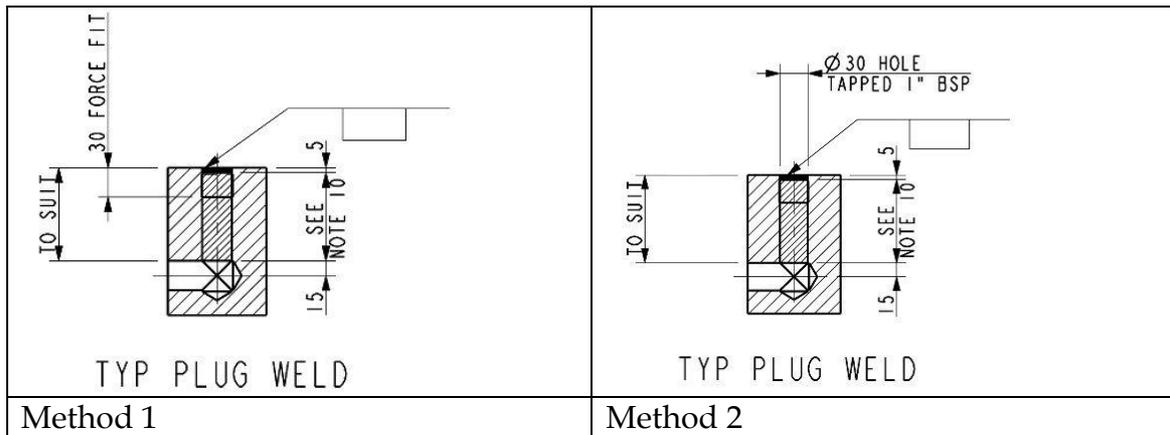
Figure 8: Plugging technique for drilled water passages
