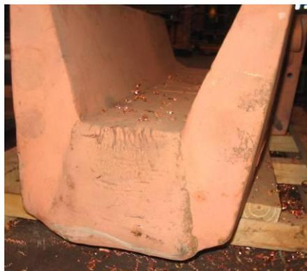
Figure 6: Repaired launder tip that originally had the rounded launder edge
