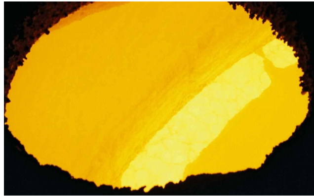
Figure 6: Vigorous boil against waffle coolers – Chambishi
