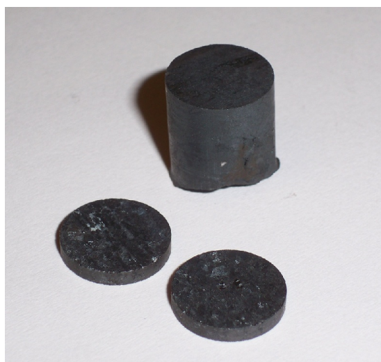
Figure 4: Assmang drilled core and disc-shaped samples (12 mm in diameter)
