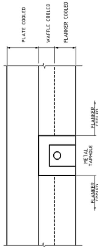
Figure 2-3: Metal taphole with flanker and waffle coolers adjacent to and above the taphole
