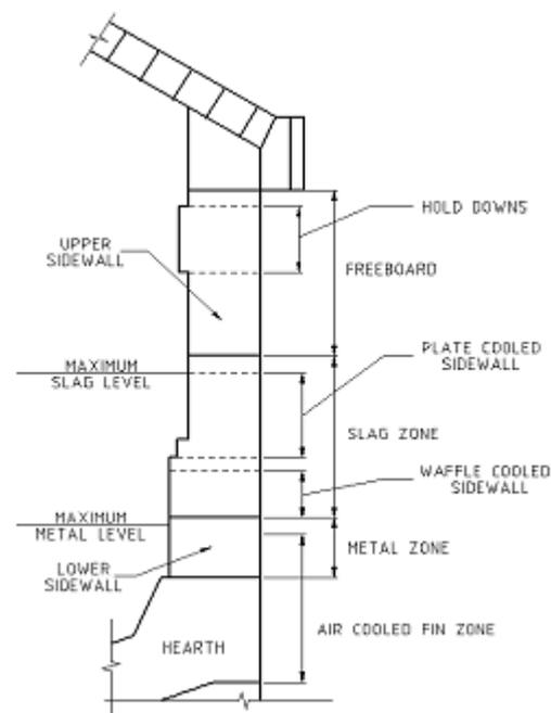
Figure 2-1: Typical Cross Section Schematic Through Furnace Sidewall
