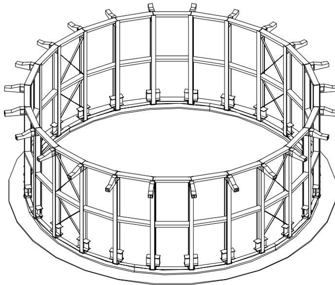
Figure 3-1: Temporary Furnace Cover Support System - Complete System (Note Shell Not Shown For Clarity)
