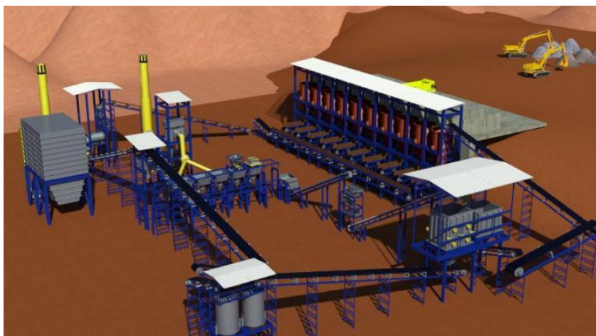
Figure 67: Mini sinter plant, typical layout
