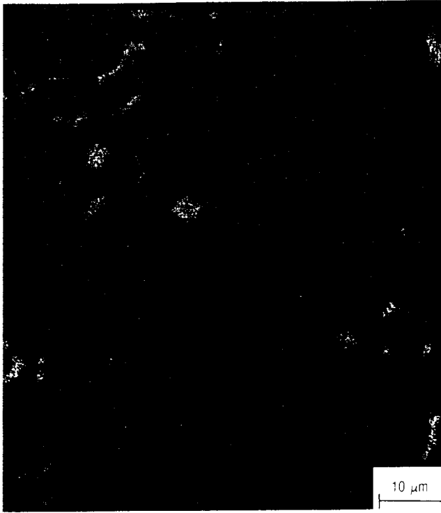
Fig. 8 — Characteristic X-ray image of the magnesia-stabilized zirconia electrolyte from Nippon showing the distribution of magnesium.
