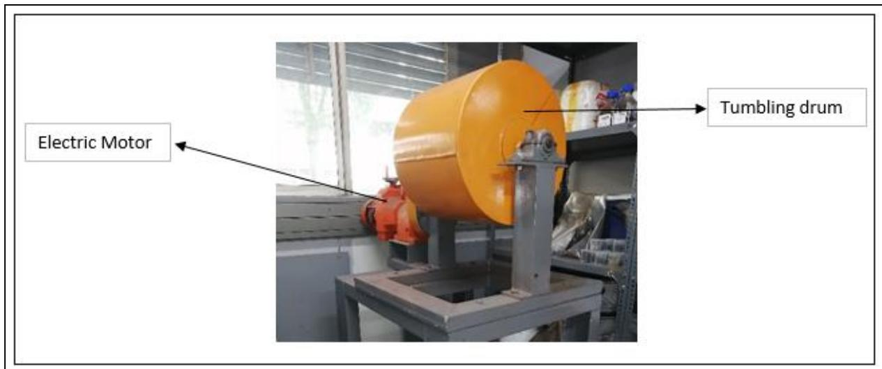
Figure 2: A picture of a tumbling drum that will be used for the test
