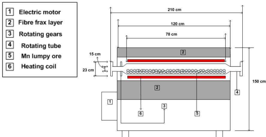
Figure 1: Experimental set-up of a rotatory kiln.
