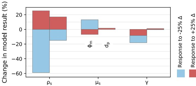
**Fig. 5** Sensitivity of model to material properties (in each group the left column indicates relative change in alloy fraction  $\phi_m$  in outlet stream, right column relative change in average droplet diameter  $d_p$ ). (Color figure online)
