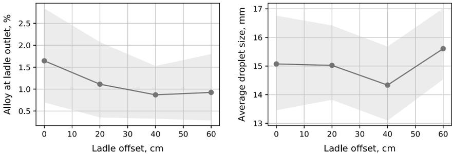
**Fig. 8** Effect of ladle lateral offset relative to inlet stream (grey bands show 90% interval)
