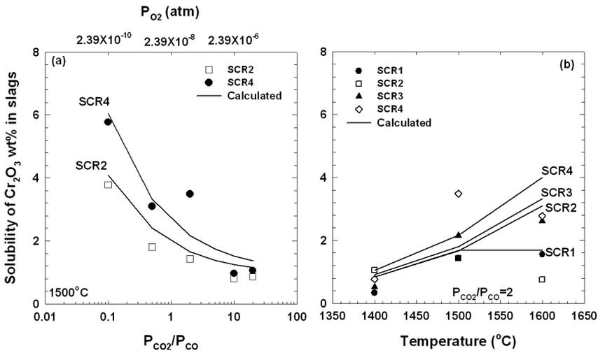
Figure 3: Comparison between the experimental data [1] and the MPE calculations on solubility of Cr as functions of (a) oxygen partial pressure, at 1500°C and (b) temperature, at  $P_{CO_2}/P_{CO}=2$  in melter type slags
