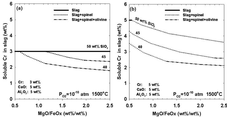
Figure 5: Effects of silica content on solubility of Cr in the slag phase as functions of MgO/FeO ratio of the melter type slags with initial (a) 3wt% Cr and (b) 5wt% Cr at  $P_{O_2}=10^{-10}$  atm at  $1500^\circ\text{C}$
