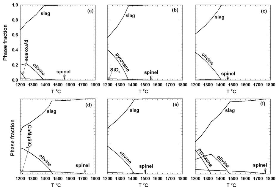
Figure 1: Calculated phase distributions as a function of temperature for the South African melter slags ((a) for S1, (b) for S2, (c) for S3, (d) for S4, (e) for S5 and (e) for S6)
