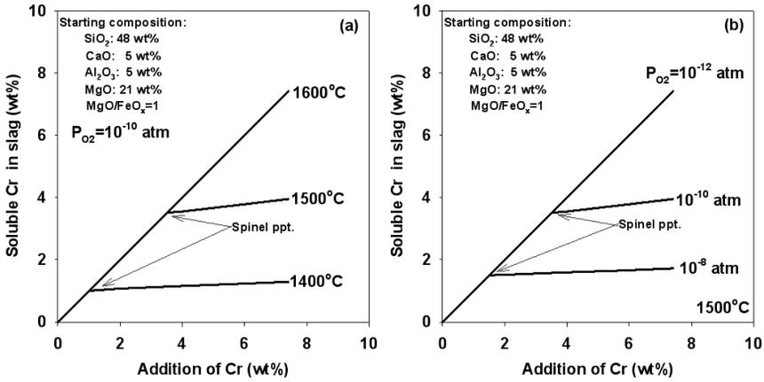
Figure 4: (a) Model predictions of the effect of temperature on solubility of Cr in the slag phase  $P_{O_2}=10^{-10}$  atm, and (b) the effect of oxygen partial pressure on the solubility of Cr in the slag phase at  $1500^\circ\text{C}$
