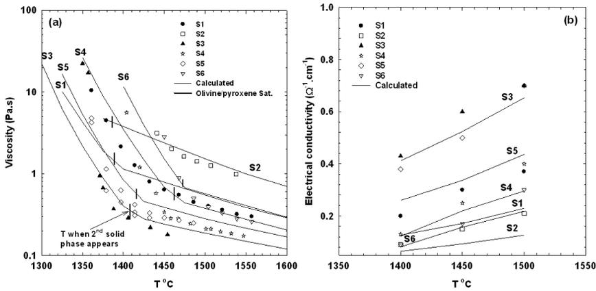
Figure 2: Comparison between the calculated and the measured (a) viscosity [11] and (b) electrical conductivity as a function of temperature for the supplied South African melter slags
